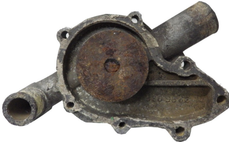
Coolant degradation / Corrosion
