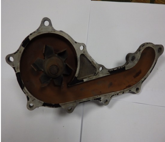
Corrosion of coolant
